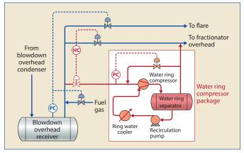
Figure 3 Water ring compressor implementation
