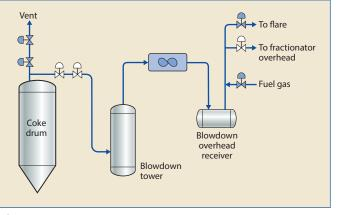
Figure 1 Traditional system with blowdown vapour routed to fractionator overhead
