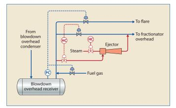
Figure 2 Ejector implementation
